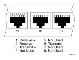
Figure 2-1. RJ45 Network Ports
